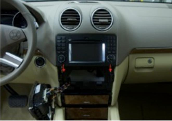
5) Pull down on retaining bars
