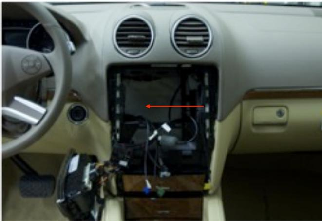
7) Access EIS wiring through opening
